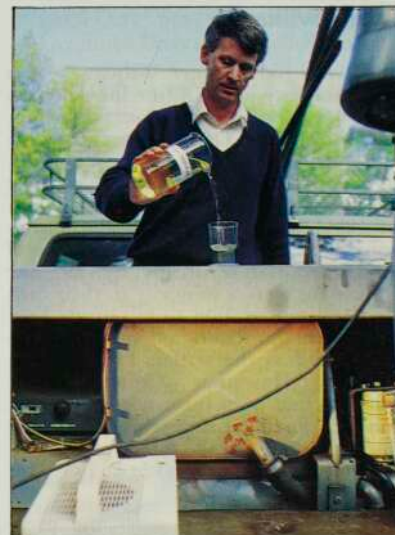
Dr David Hagen: pouring coconut oil into a diesel-powered generator
