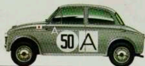
1962 Mitsubishi 500 First of its class in the Macao Grand Prix. Powered by an air-cooled two-cylinder engine generating 21 ps.
