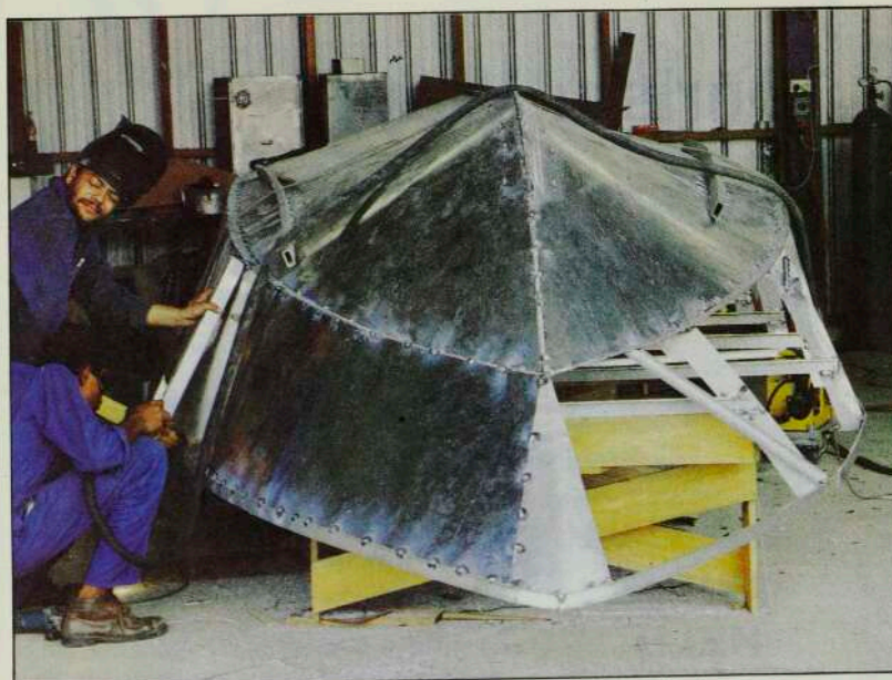
Special: an aluminium fishing boat being built Fiji Customs Craft
