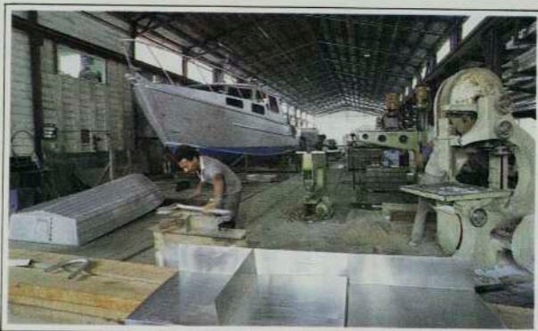
Interior workshop showing Aluminium Catamaran under construction.
