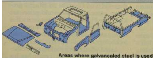
Areas where galvanealed steel is used
