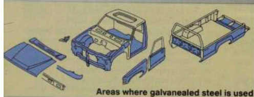
Areas where galvanized steel is used
