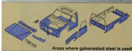
Areas where galvanized steel is used
