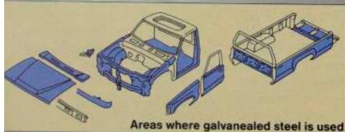
Areas where galvanized steel is used
