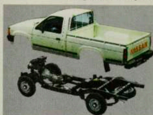
The Nissan Pickup's ladder frame and body are built for extra strength.
