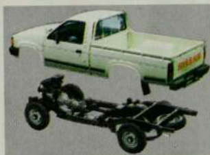
The Nissan Pickup's frame and body are built for extra strength.
