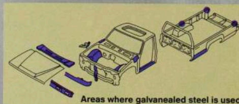
Areas where galvanealed steel is used
