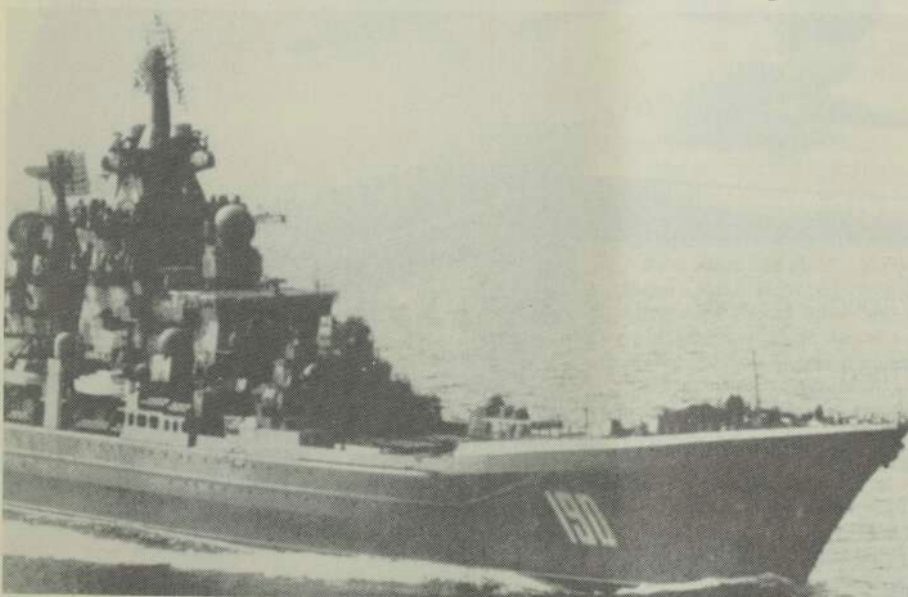
The nuclear-powered guided-missile cruiser FRUNZE, second unit of the KIROV-Class, at 28,000-tons displacement, is 248 meters in length, carries RBU-6000 rocket launchers, 96 vertically launched SA-N-6 surface-to-air missiles, and 20 SS-N-19 surface-to-surface missiles as well as ADMG Gatling guns on its foredeck.
