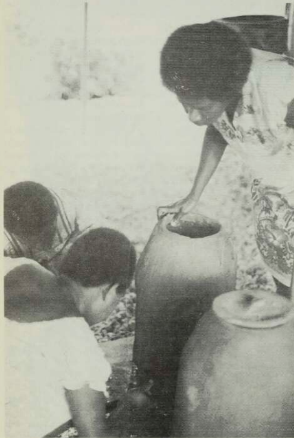
Girls at the Onesua Community Education Centre in Vanuatu learn to make cement water jars. Photo: D. Goodwillie.
