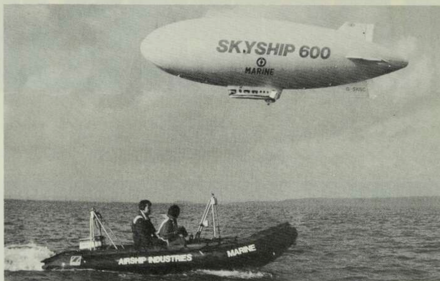
Fast inboard-outboard rigid inflatable boat carried under the Airship allows direct inspection of suspect trawlers.
