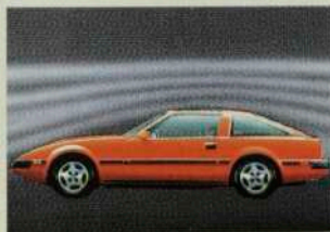
The Nissan 300ZX achieves one of the lowest drag coefficients ever—0.31.
