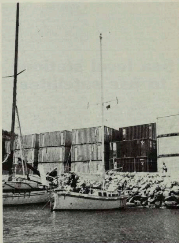
Atoll , based on a riveted alloy lifeboat hull, at anchor in Port Moresby.
