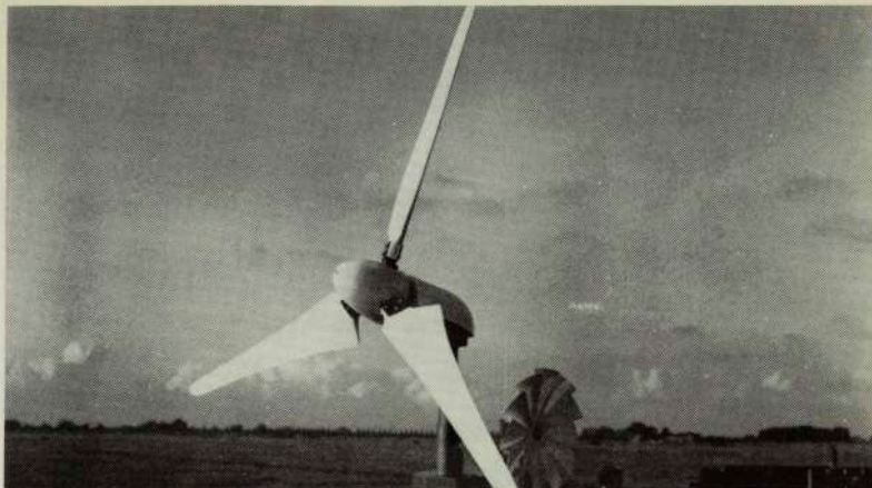
The Dutch were building windmills 600 years before the invention of the steam engine. This is one of their latest, and most efficient, the Longlife LMW generator which produces 1000 watts of power, for a capital cost of less than $A3000.
