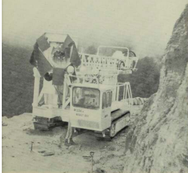
A long way to the bottom: This Driltech crawler-mounted chip-sampler is now operating high in the mountains of Papua New Guinea as part of the Ok Tedi copper and gold mine development. The unit was shipped from Australia, taken across the Gulf of Papua by barge from Port Moresby to Kiunga, carried inland on a low loader over bush tracks, and then driven under its own power over Mount Fubilan to begin chip sampling. Sullair Australia Ltd. supplied the unit.
