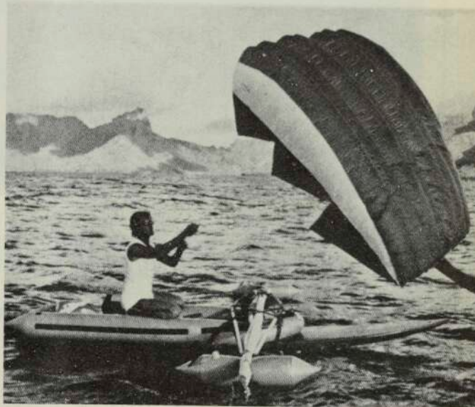
The picture reveals how Arnaud de Rosnay did it. Thanks to the inflated rubber gunwale, the surfboard is transformed into a small zodiac dinghy. The mast is securely tied across the craft, and, equipped as it is with plastic floats on both sides, it acts like a double canoe outrigger boom. The whole strange contraption is pulled by a huge inflatable kite. In this manner great safety and stability are achieved at the expense of speed. Actually the average speed for de Rosnay's 10-day cruise was only two knots. — Paris-Match picture
