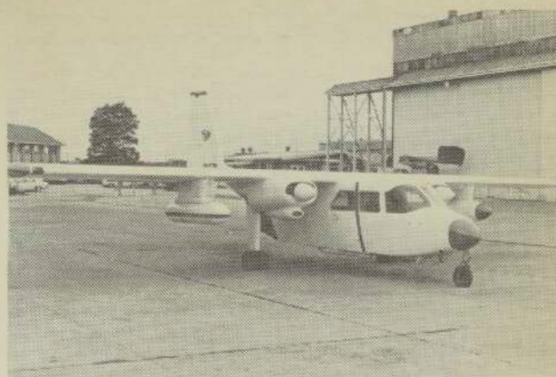
A Britten Norman Islander with the de Havilland surveillance pod fitted under its starboard wing.
