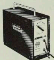
Lincoln Jetwelder 130 , portable transformer welder; welding range 45 to 130 amps AC. Operates from 240 volts AC mains supply. Handles electrodes from 2mm ( \frac{1}{16} " ) to 3.15mm ( \frac{1}{8} " ).
