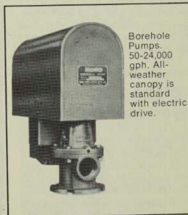
'E' type Borehole Pump. Close- coupled. 0.75 hp elec. motor. 410- 1,560 gph; depths to 150 ft.
