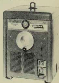
Lincoln TM heavy duty transformer and transformer/rectifier welders—range of six models for AC and AC/DC welding up to 750 amp, handling electrodes in the range 2.5 to 10 mm ( \frac{1}{8} " to \frac{3}{8} ") for all models. Input power 415 V 50 Hz single phase. Special voltages can be supplied.
