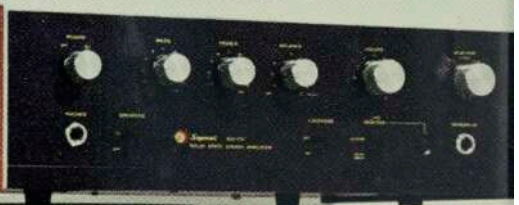
AU-101 18/18 Watts, Distortion (max.): 0.4%
