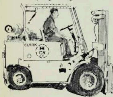
FORKLIFTS. Seven custom-designed forklift trucks with triple stage masts and side shift carriages are permanently garaged on board for the safe, mechanised handling of your cargo.
