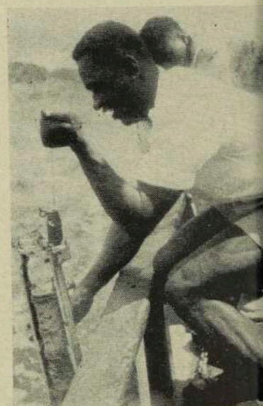
Outside Suva Harbour Fijian Joeli Romanin covers the reversing-bottle with its side of sea water from 75 fathoms.
