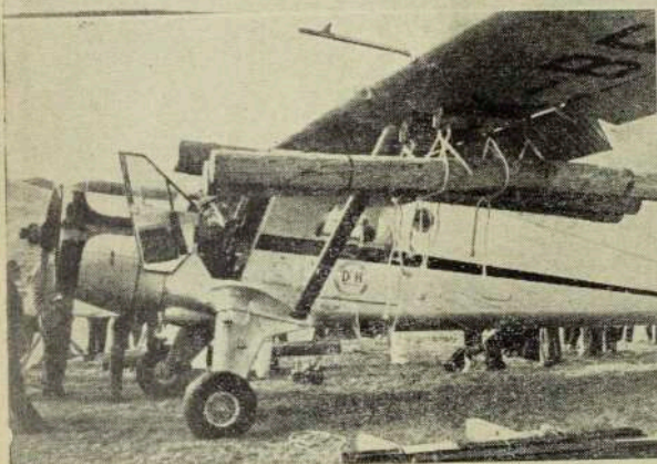
THE BEAVER SHOWING WING ATTACHMENTS Posts for building stockyards are shown being carried on supply-dropping racks of a De Havilland Beaver. The posts are 11 ft. long and 8 in. in diameter and weigh approximately 130 lb. each.
