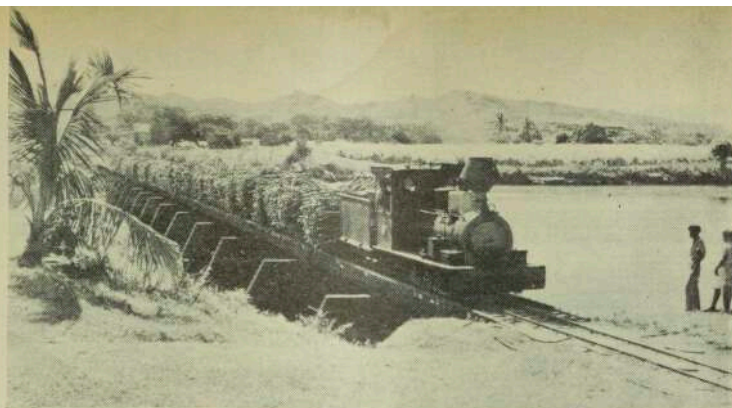
A locomotive brings a long rake of cane trucks to the CSR's Rarawai mill. The com- pany has about 400 miles of light train line altogether; this section is about 180 miles long and passengers are carried free.
