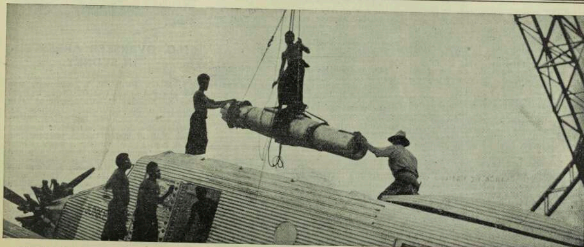
The heaviest load ever carried in from the coast to the goldfield in New Guinea. Tumbler shaft for new dredge, weighing 7900 lbs., being unloaded from G31 aeroplane, operated by Guinea Airways Ltd.
